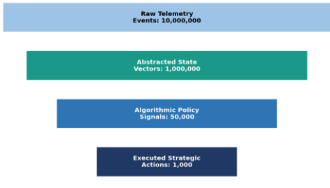
Figure 14. Raw telemetry enters the top of the funnel at peak volume , where initial edge filters immediately discard redundant noise and structural anomalies. The intermediate streaming layer then aggregates high-frequency bursts into structured event windows, achieving an order-of-magnitude reduction in data throughput. Sub-second decision engines evaluate these refined event streams against active operational rules to distill high-value execution triggers. Ultimately, only highly validated, context-rich signals pass through to final execution, ensuring system resources target high-impact business events without platform overload.
