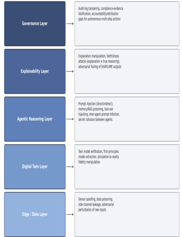
Figure 2: Representative attack surface mapped to each layer of the proposed architecture.
